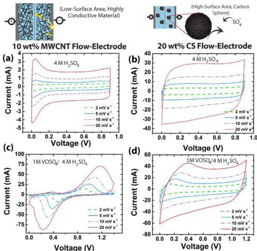
**Figure 2.** Cyclic voltammograms for flow-electrodes based on nanoscale (MWCNTs) (a) and microscale (CSs) conductive carbon particles (b) in sulfuric acid. CVs are transformed when a  $\text{VO}^{2+}/\text{VO}_2^+$  redox couple is introduced into the flow-electrodes based on MWCNTs (c) and CSs (d).
