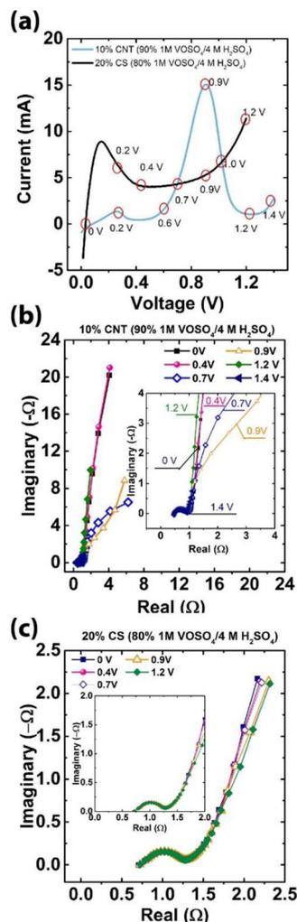
**Figure 4.** Representative shapes of cathodic curves at  $2 \text{ mV s}^{-1}$  for flow-electrodes based on the  $\text{VO}^{2+}/\text{VO}_2^+$  redox couple (a). PEIS at different voltages for the MWCNT (b) and CS (c) based flow-electrodes.
