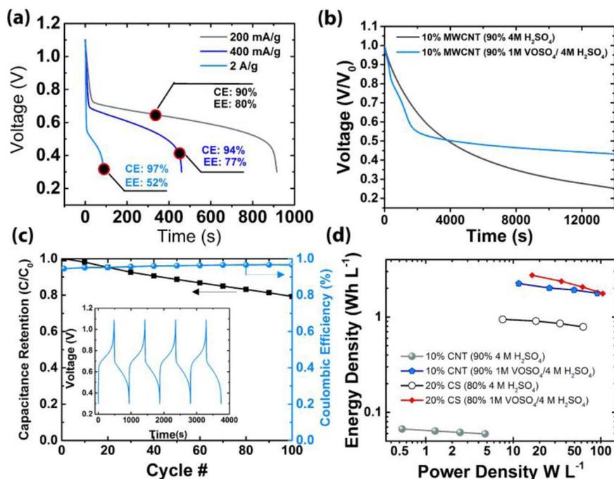
**Figure 5.** Representative galvanostatic discharge curves at different rates (a), self-discharge (b), cycle life, and coulombic efficiencies at a charge rate of  $400 \text{ mA g}^{-1}$  (c), and Ragone plot from cyclic voltammetry data in Fig. 2 (d).
